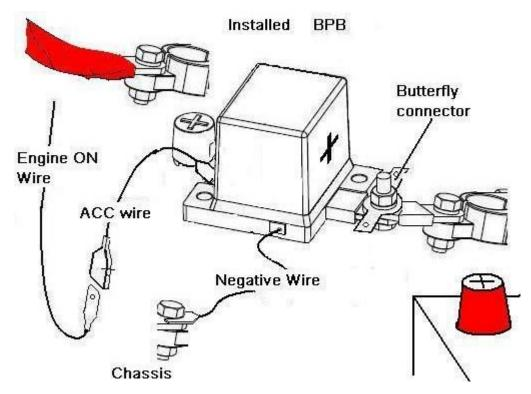
To bypass the BPB, connect the ACC wire to the butterfly connector.
